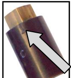
Bad Brush Holder (photos and illustration) – Look for scarring or marking on the surface of the carbon brush holder. These may be electrical shorts.
